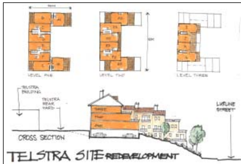
Three Floor Plans and Building Section of Proposed Design for Rear of Telstra Property
